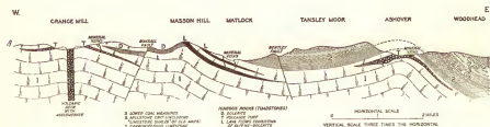
FIG. 12.—Section across the eastern part of the Derbyshire Dome, illustrating the occurrence of toadstones.
